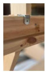
Using the two ladder hooks now attach to the top of each ladder strut, attaching to the slanted inside cut edge, See PIC1 Locate the hooks and attach using the small screw(L). Now hook the ladder over the side rail, this is designed to be tight to prevent movement. You may need to gently tap with a mallet..
