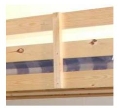
These two rails prevent the guard rails from being forced apart, very important. Using a tape measure find the centre of the back guard rail and centre of the front guard rail. Make a small pencil mark. Then attach each guard rail support to the front using base slat screw (E) provided. These cover both the two guard rails and secure onto the side rail.
