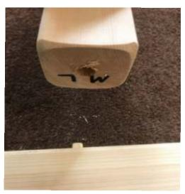
We now need to attach the bottom headboard facia 4E. You will note this has a dowel hole on the top, please locate a wooden dowel. This now connects to the bottom of corner post ML.
