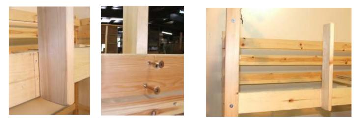
Now find part 11A, you will note this has no pilot holes. Line the part 11A to the mark made on the side rail, the 40cm is the minimum gap so line up furthest away from your mark.
