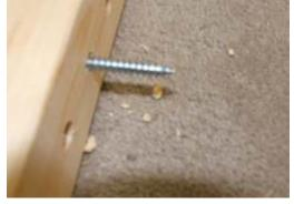
BEFORE you start assembly clear these holes with one of the bolts. Push the bolt through each hole, this will dislodge any sawdust or debris that could interfere with fixing the bed.
