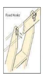
Using the two ladder hooks now attach to the top of each ladder strut, attaching to the slanted inside cut edge, See PIC1 Locate the hooks and attach using the small screw(L). Now hook the ladder over the side rail, this is designed to be tight to prevent movement. You may need to gently tap with a mallet..
