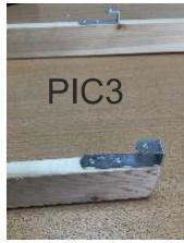
Now we have assembled the ladder we need to attach the hooks. If the ladder is going on the right side lay the ladder on the carpet as shown in PIC2, if left lay as shown in PIC1. (Note the position of the long strut). We are attaching two ladder hooks at the top. Now place a pencil mark 320mm down from the top of the long ladder strut. (PIC4, see A), the second hook goes at the very top of the small strut. Then position the ladder hook to these marks and attach using small screw(L) (PIC3)
