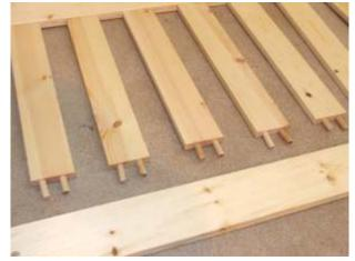
Lay two headboard facias marked Black PART 9 (4G) position these as shown in PIC 1. Lay the long inserts (PART 12) in between these ready to join.
